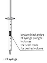
6. Place the syringe with the Reagent Mg-2 in the hole cap. Press the MEAS key and begin the titration by carefully adding Reagent Mg-2 in small portions. If the entire volume of the syringe is emptied and there is no end of titration, take another portion (1 ml) of Reagent Mg-2 and continue titration.
